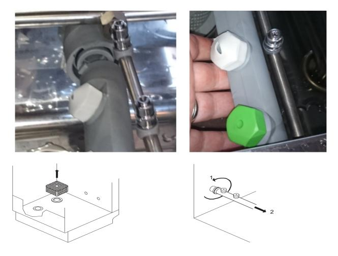
Take off the pump filter and the surface filter and rinse them under flowing water. Take out the rinsing arms by slightly turning them to the left.
