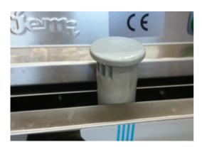
Insert the overflow pipe into the door frame, so that the interior may "air".
