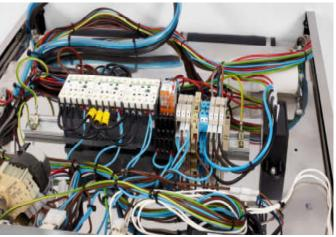
The whole technology of the bottle washing machine is electromechanical. No electronics or boards included. Hence it is easy to handle and malfunctions can be remedied rapidly.
