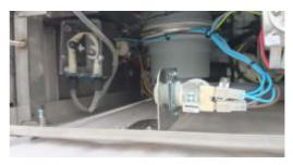
The new booster pump guarantees optimum fresh water rinsing after the washing cycle.
