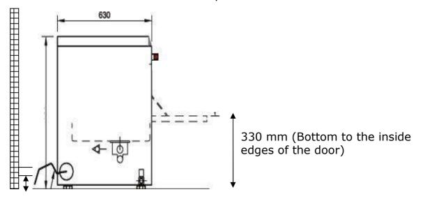
Water drain 50-60 mm from the floor Machine height 820 mm
