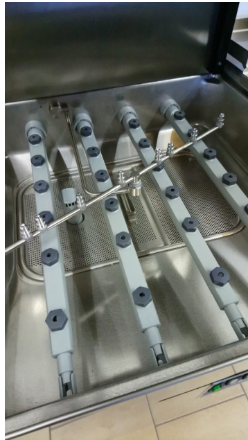
Rinsing arms for the rinsing of yoghurt jars, work utensils, crates or buckets, etc.
