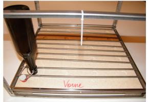
Important: Always check the position of the bottle mouth, in order that it is exactly positioned with the recess of the template.
