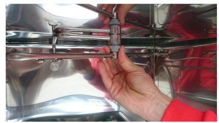
Insert the Allen screw included in the delivery into the thread; do not overtighten it.
