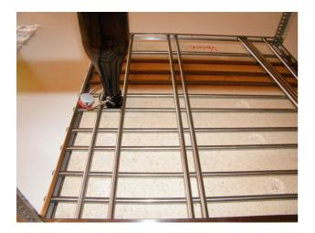
Always check the exact position of the bottle mouth with the recess of the template.
