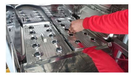
Remove the upper rinsing arm by turning the grey plastic nut.
